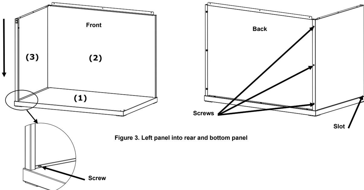
Figure 3. Left panel into rear and bottom panel
