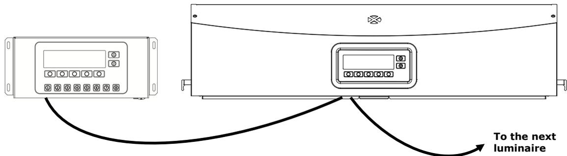
4. Continue connecting daisy chain cables to the remaining luminaires (left port in and right port out).
